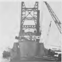
BUSINESS END of the Queen of Holland NAP's 3,000,000 dredge belonging to the Amsterdam Ballast Company, is the big rock cutter. ESAKI TA a punto fuerte di Queen of Holland, e draga NAP's 3,000,000, cual ta propiedad di Amsterdamse Ballast Maatschappij. Esaki ta a cortador.
